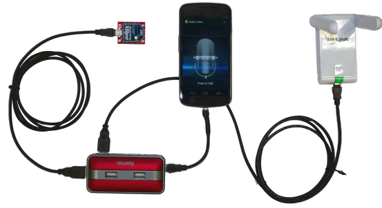
Figure 5: Walkie Talkie app (cf. Section 5.2) on prototype with external 802.11 and 802.15.4 radios.
